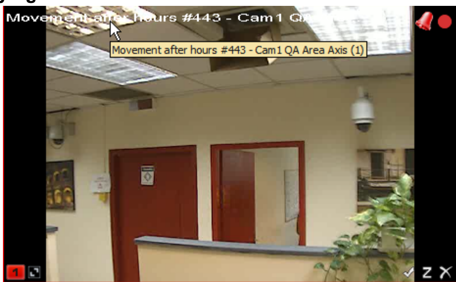
OSD text and icons indicate what alarm and which of the alarms cameras is now displaying
