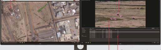
Events automatically created in VMS upon radar detection and target classification
